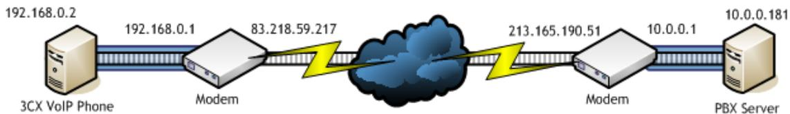
Figure 4 - How a tunnel works
