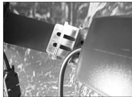
Picture 4: Slide RDU into the mounting slider
