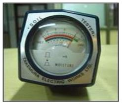
Fig. 5 Soil Moisture and pH Sensor
