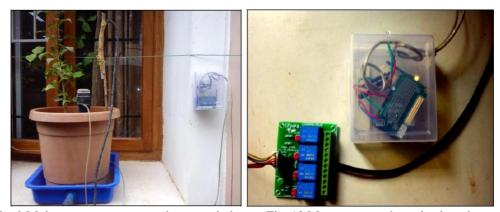
Fig. 9 Moisture sensor connected to potted plant Fig. 10 Mote connected to relay board
