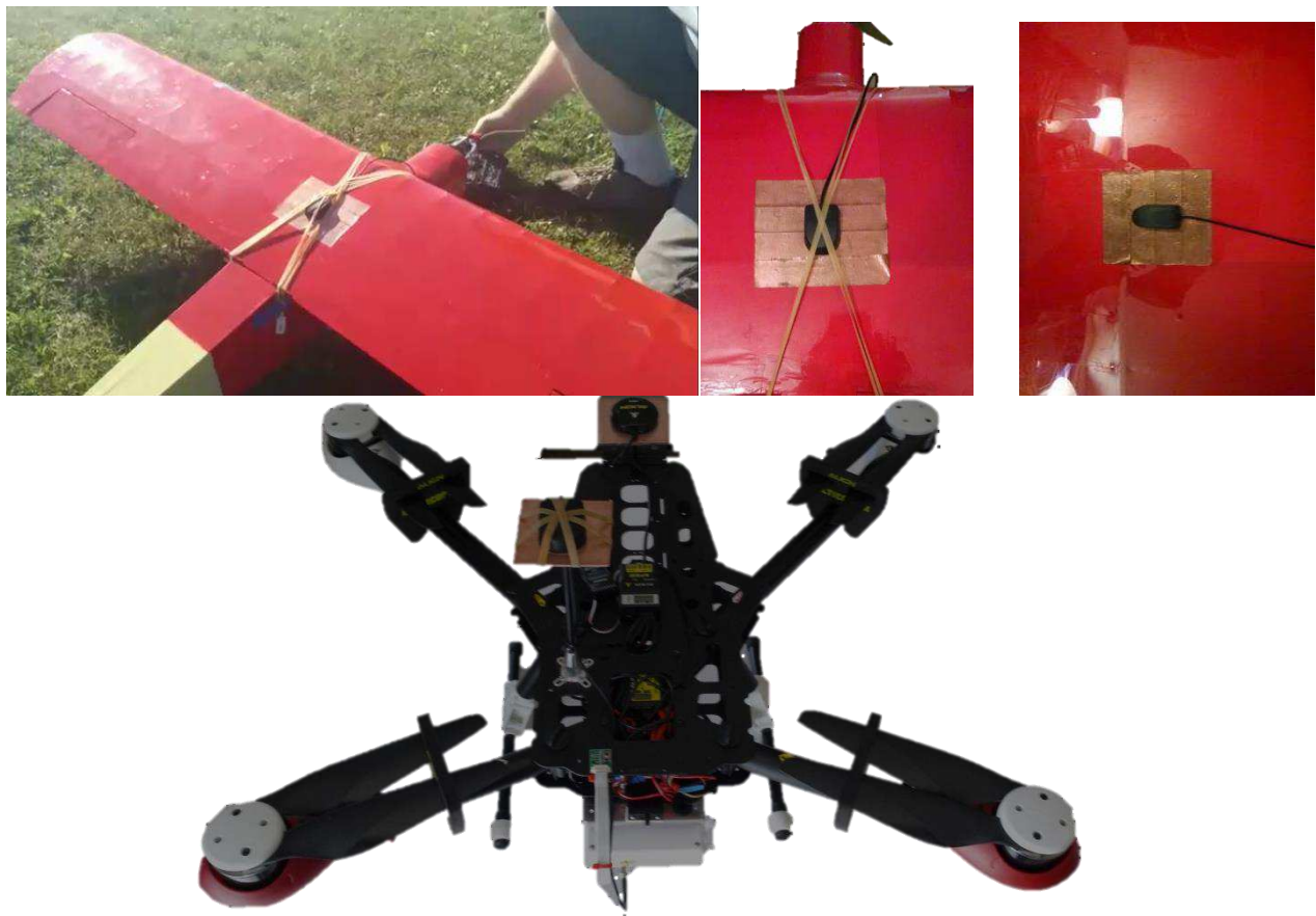
Figure 7 Example of proper antenna install on ground plane (copper tape) on center topside of plane or quad away from other electronics.
