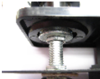
Nuts/Washers Installed Between L Bracket and Faceplate
