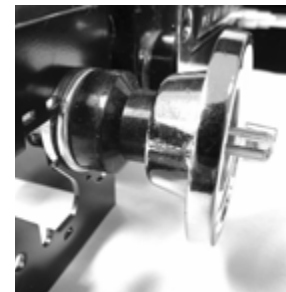
Figure 5 - Shaft Cover Installed
