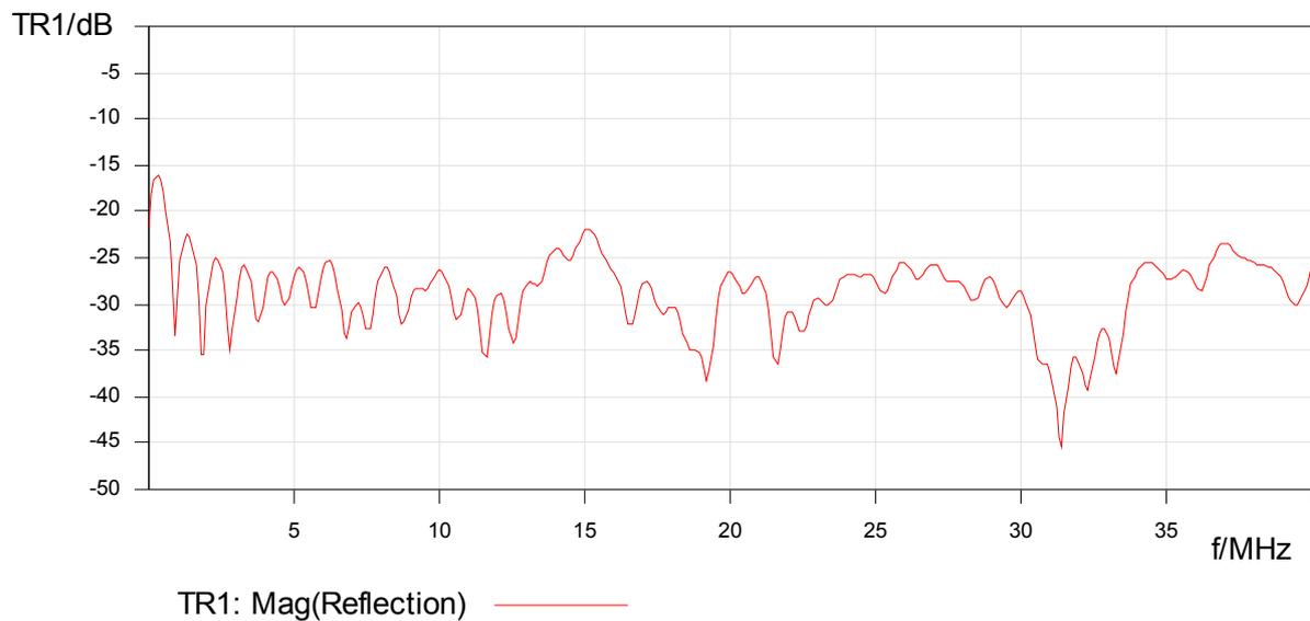
**Result:** The ripple of the return loss is caused by cable deflections.
