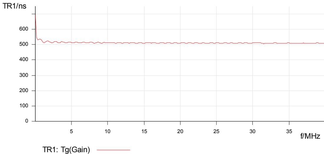
**Result:** The group delay is around 500ns for 100m cable – this is approx. 5ns/1m. It is also possible to calculate the propagation speed like shown in the next section.
