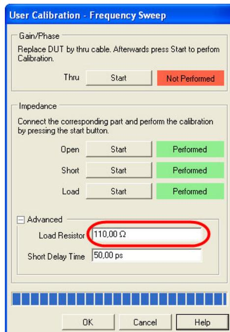
**Note:** Perform the different impedance calibration modes with an open/short/load connector as described in the User Manual.
