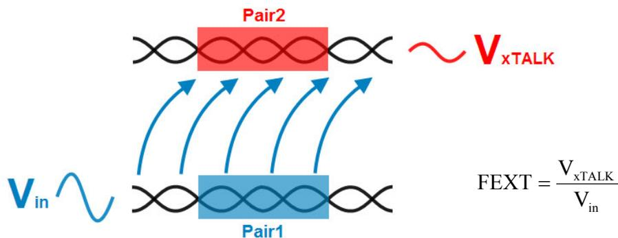
**Hint:** Far end crosstalk can also be expressed as Equal Level Far End Crosstalk (ELFEXT), which is calculated. ELFEXT is FEXT measured with respect to the attenuated test signal (see Add-On "ELFEXT Measurement with Bode 100").
