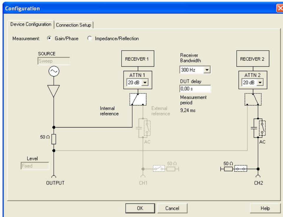
To minimize the influence of the BALUNs and cables used to connect the DUT to Bode 100 it is advisable to perform a THRU calibration as shown in the manual in the section "Calibration in the Gain/Phase mode".
