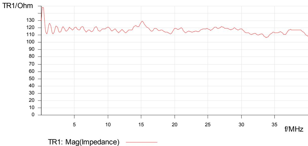
**Result:** As we can see, the impedance of our DSL-Cable has a slight deviation from the ideal Load (110 ohm). The reason is that the wave resistance of our DSL-Cable, which is 120 ohm. The ripple is caused by variations and deflections in the cable construction.
