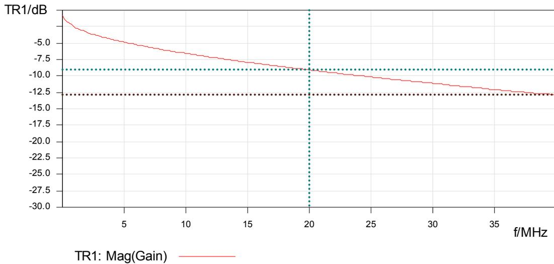
**Result:** The maximum attenuation at 40MHz is about 12,9dB/100m (for information on setting the cursors see the Bode 100 User Manual). The attenuation at 20 MHz is about 9dB/100m.
