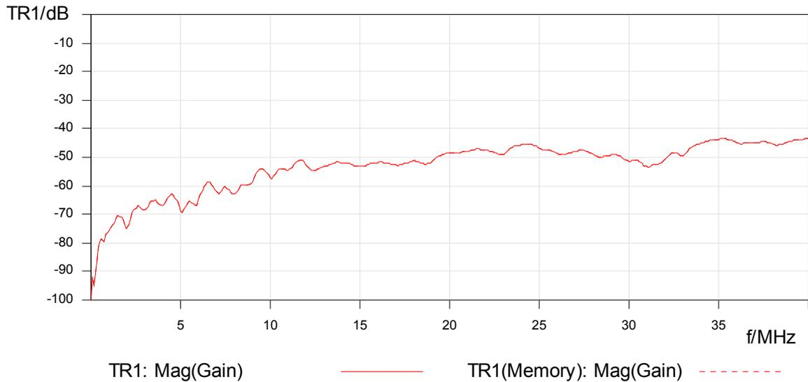
This graph shows the crosstalk (NEXT) between two neighbouring pairs. Our measurement result shows that the signal received at the near end of Pair2 is -40dB or more below the signal sent into Pair1.
