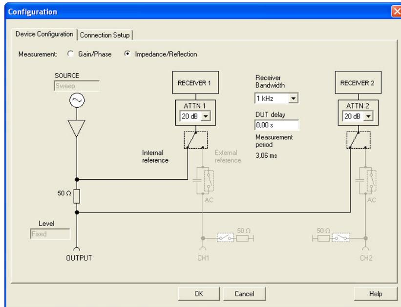
For the impedance measurement you have to set the load resistor to 110 ohm in the advanced settings of the calibration window.
