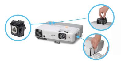
Longer lamp life enables customers to extend maintenance cycles to up to 6000H.
