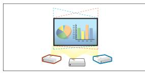
These projectors provide vertical (automatic/manual) and horizontal (manual) keystone correction. Thanks to these functions, it is not necessary to put the projector in the center of the desk. You can place the projector anywhere you want.
