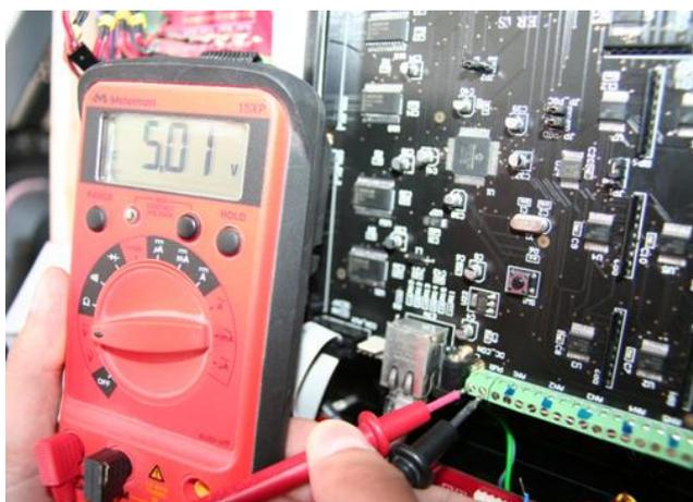
To configure the Board, and once the connection to the control computer is made, directly or by means of a Switch or Hub, proceed to supply externally the Ethernet SC-MMB Mother Board.
