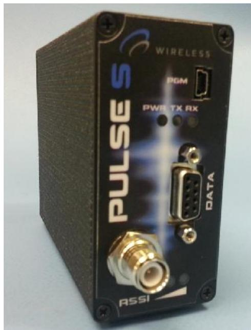
The PULSE 'S' is equipped with a standard RS232 DB9 connector, which you connect to your serial device. Data from your serial device is transparently sent to other ENCOM PULSE Wireless Modems using license free 900 MHz technology. LED indicators on the front panel provide serial and RF status information.
