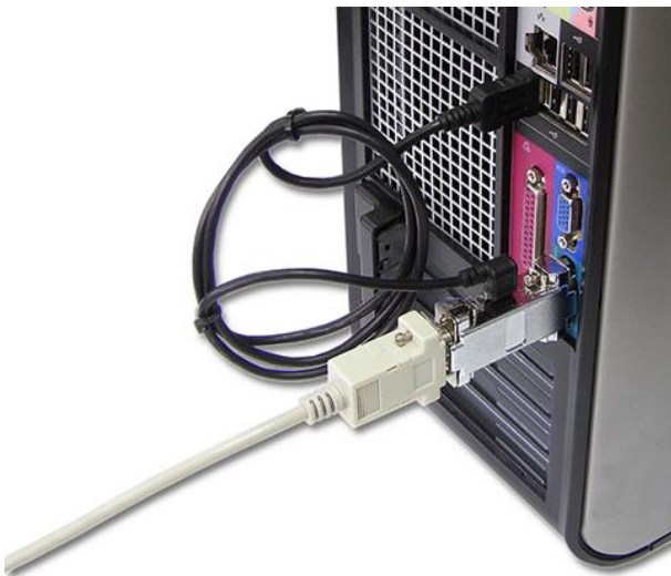
SerialGhost in record mode powered from a USB port.
