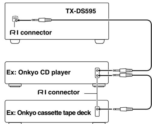
To connect components using the **RI** terminal, simply connect a remote control cable from this **RI** terminal to the **RI** terminal of the other component. An **RI** remote control cable with a 1/8-inch (3.5-mm) miniature two-conductor plug comes with every cassette tape deck, compact disc player, MD recorder, and DVD player that has an **RI** terminal.
