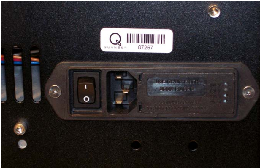
Figure 4 Fuse on back panel of UPM-15-03/UPM-24-05.
