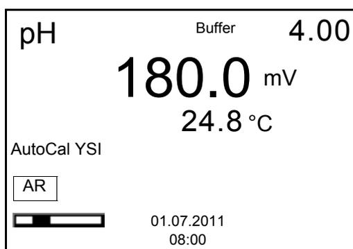
18. Wait for the measurement with stability control to be completed or terminate the stability control and take over the calibration value with **<MENU/ENTER>**.
