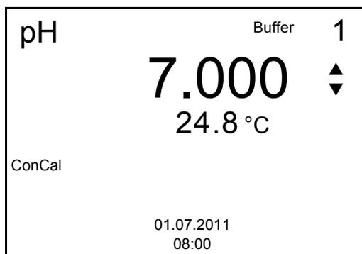
8. Set the nominal buffer value for the measured temperature with **<▲><▼>**.
