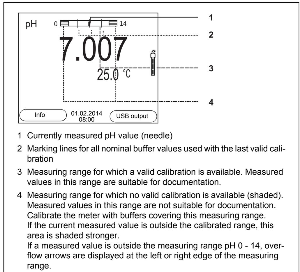
The limits of the calibrated range are determined by the buffers used for calibration:
