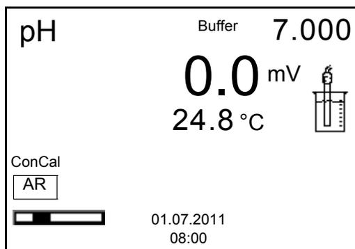
7. Wait for the measurement with stability control to be completed or terminate the stability control and take over the calibration value with **<MENU/ENTER>**.
