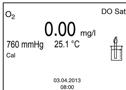
7. Put the IDS D.O. sensor into the calibration medium.
