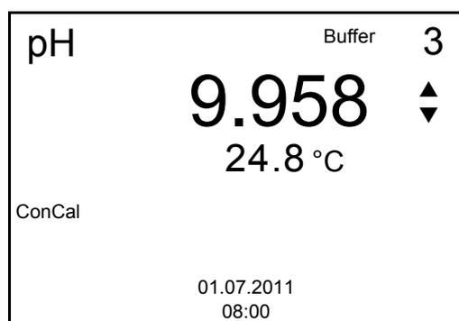
22. Set the nominal buffer value for the measured temperature with  $\langle \blacktriangle \rangle \langle \blacktriangledown \rangle$ .
