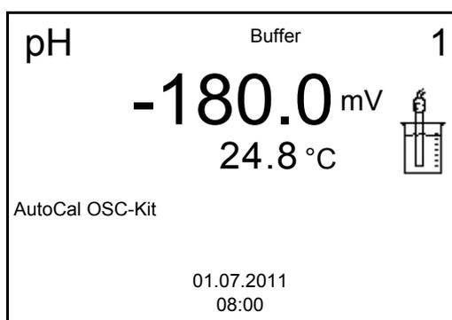
3. Calibration with the buffers of the QSC-Kit is done like a normal three-point calibration.
