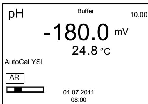
7. Wait for the end of the measurement with stability control or accept the calibration value with **<MENU/ENTER>**.
