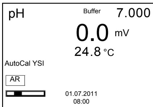
13. Wait for the measurement with stability control to be completed or terminate the stability control and take over the calibration value with **<MENU/ENTER>**.
