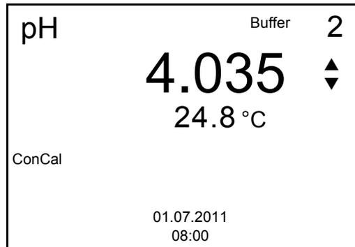
15. Set the nominal buffer value for the measured temperature with **<▲><▼>**.
