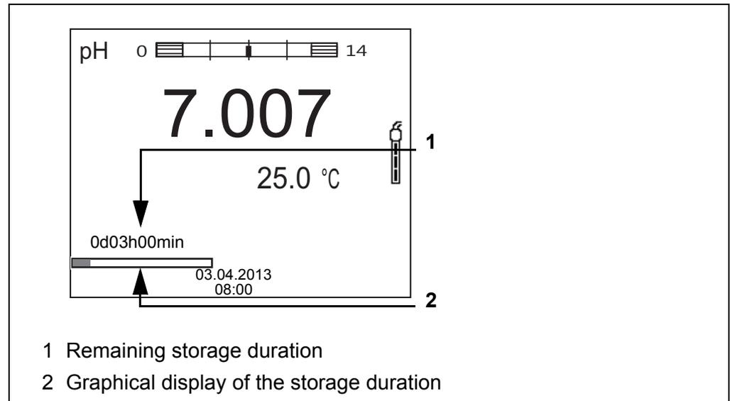
The active automatic data storage function can be recognized by the progress bar in the status line. The progress bar indicates the remaining storage duration.
