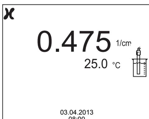
4. Immerse the conductivity sensor in the control standard solution, 0.01 mol/l KCl.
