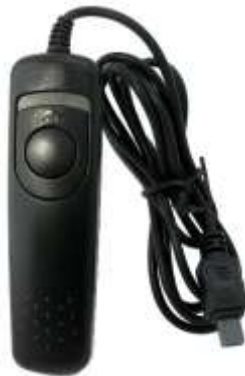
A corded remote shutter release like this one can be rewired to work on two cameras at the same time
