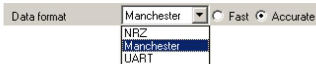
The selection between Fast and Accurate controls the settling time of the averaging filter in the demodulator. Please see the data sheet for details.
