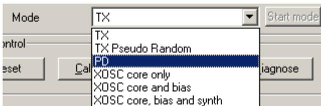
If pseudo random sequence is selected, the DI is XOR'ed with this predefined sequence in TX. The pseudo random sequence in TX mode is initiated by a negative transition on PSEL. Pushing the 'Start PN9' button does this.
