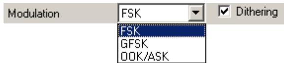
In a fractional-N synthesizer, spurious signals can occur at certain frequencies depending on the division ratios in the PLL. To reduce the strength of these spurs the Dithering can be enabled.
