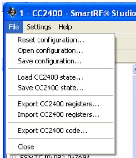
*Reset configuration*- This command will reset all fields in SmartRF® Studio. The connected device is not affected. The command is also available from the toolbar (white sheet).
