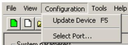
The configuration menu allows you to change port address or device, and download the data to the device.
