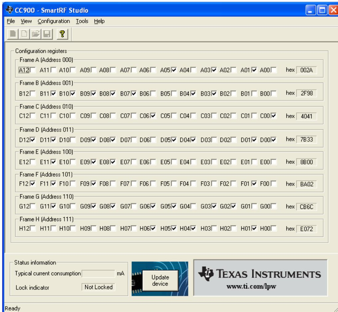
In this mode you can change the 13 different bits in the 8 registers directly by clicking on the white squares. These bits are used to program the transceiver chip on the printed circuit board (PCB) that follows Development Kit. We dissuade you to change the bits without contacting our company first.
