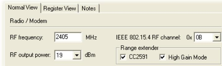
The Range extender mode is only applicable with the CC2591 and CC2590 Combo Board. The Combo Board is an Evaluation Module that combines both a CC2520 and the front end CC2591 or CC2590.
