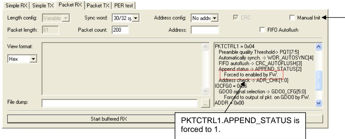
This means that the user will not be able to change these values. If the user enters the Register View and change PKTCTRL1.APPEND\_STATUS to 0 and check the “Manual Init” box, this value will be overwritten by the FW when “buffered RX” is started.
