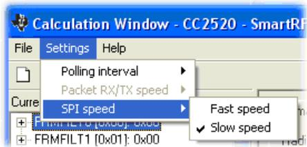
*SPI speed* - Defines the SPI communication speed between the USB MCU on SmartRF® 05 evaluation board and CC2520.
