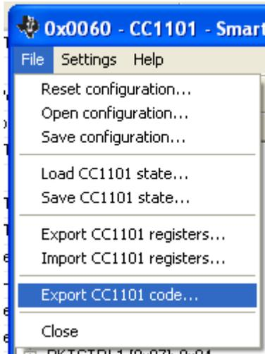
*Reset configuration*- This command will reset all fields in SmartRF® Studio. The connected device is not affected. The command is also available from the toolbar (white sheet).
