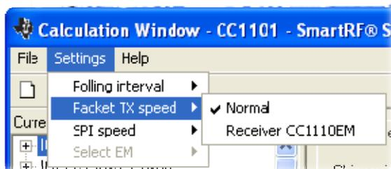
*Packet TX speed* - Sending of packets to other RF devices might require different time interval between each packet. This is due to the packet handling of SmartRF Studio. Packet TX/RX between two equal RF devices should use "Normal" setting. "Receiver CC1110EM" should be used if sending packets to a CC1110EM device.
