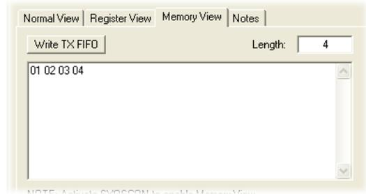
Press "Read Ram" button and see that the data has been written to the TXFIFO. See also that the length byte has been put in front of the data. Note that the length byte includes 2 bytes for the CRC that will be appended to the packet by hardware unless the default setting of "AUTOCRC" has been changed.
