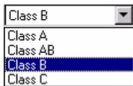
The selection of power amplifier operation class is a trade-off between output power, efficiency and harmonic generation. In class A or AB the amplifier is working more linear, and the harmonics will be low. However, the efficiency and the output power will also be low. For increased output power and efficiency, class B or C should be used, with the cost of somewhat higher harmonics.
