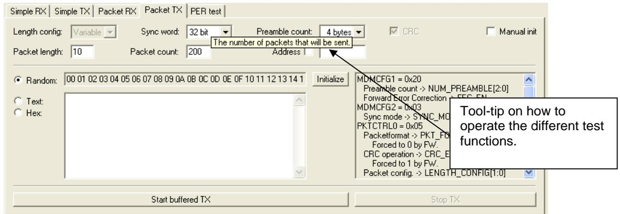
Warnings are indicated by turning the relevant control(s) yellow. One such warning will appear when choosing a sync word smaller than 32 bits in the Packet RX/TX tests in Normal View.
