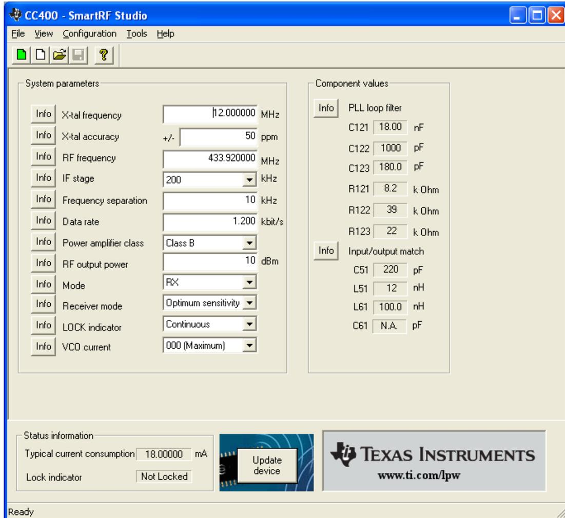
You can get information about the different parameters by clicking on the **info** button to the left of the parameter. In addition to this, a tool-tip message appears when you move the mouse over a feature.
