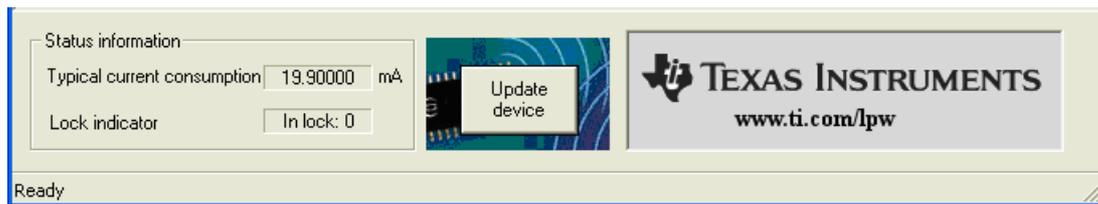
The user can observe the current consumption of the transceiver in the different settings in the Normal View. SmartRF® Studio also monitors the lock pin of the transceiver.
