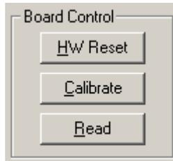
**Calibrate** activates the on-chip calibration feature of the VCO and PLL on the CC1010.
