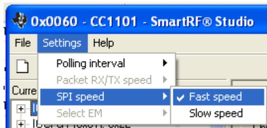
*SPI speed* - Defines the SPI communication speed between the SmartRF® 04 evaluation board and CC11xx/25xx. This option is not available for CC430.
