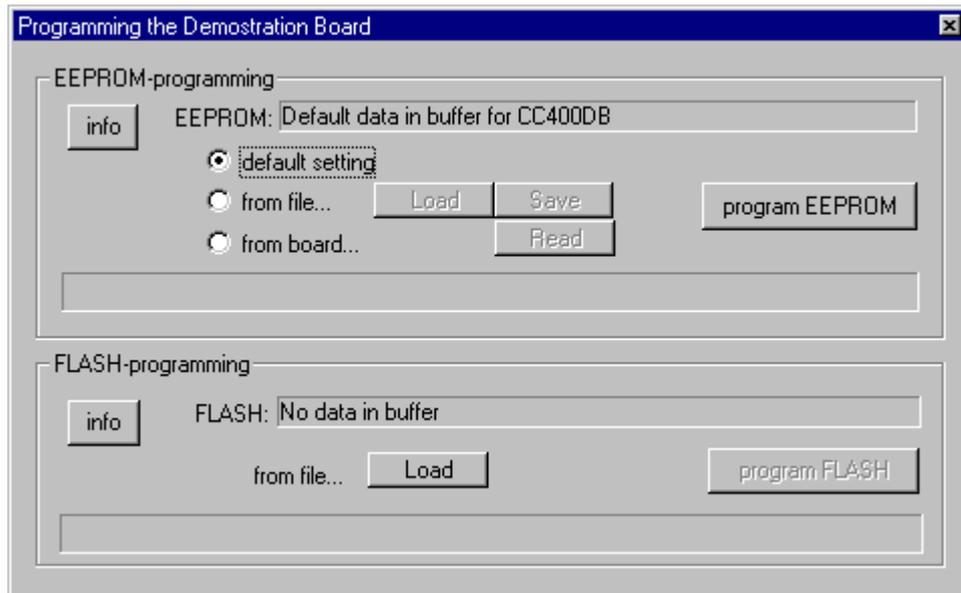
The interface communicates with the Evaluation Board. Before programming can start, you must plug the Demonstration Board into the edge connector on the CC400/900 Evaluation Board. The software will inform you if you have not installed the Demonstration Board correctly on the demonstrator before programming. Please see the User Manuals for the Development Kit for details regarding the Evaluation Board and Demonstration Board.
