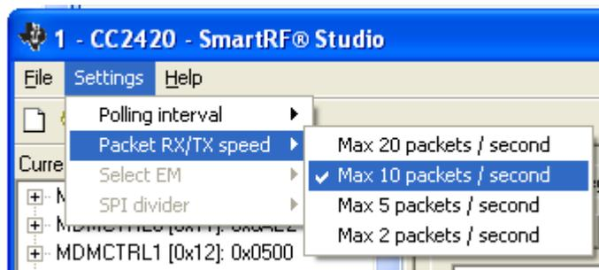
*Packet RX/TX speed* - Defines the minimum transmission interval for packet transfer in Normal View. Reduce this value in RX and TX (both!) if the number of lost packets seems unreasonably high.
