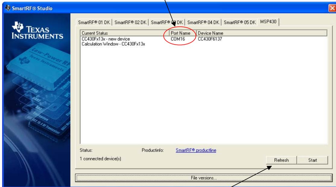
A refresh button can be used to refresh the list of connected devices
