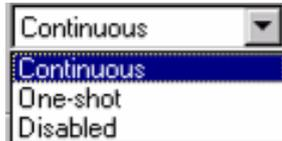
Important: The 'One-shot' lock signal is used internally in the CC900 to enable the transmitter. If the lock signal is not active (high) the transmitter will not be enabled. This is done in order to avoid the transmitter to emit out-of-band signals. If 'Disabled' is chosen this function is overridden and care should be taken, as the transmitter will transmit even when the PLL is not in lock.
