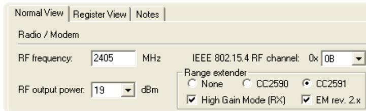
The Range extender mode is only applicable with the CC2591 and CC2590 Combo Board. The Combo Board is an Evaluation Module that combines both a CC2430 SoC and the front end CC2591 or CC2590.
