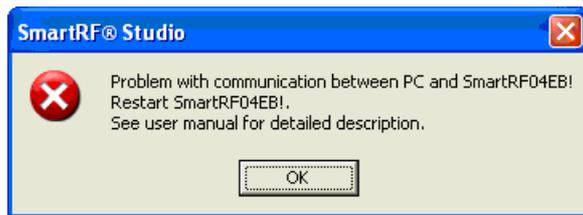
The problem is related to the use of the power switch on the SmartRF04EB board. When the switch is turned on, the boot sequence on the USB MCU will sometimes fail. One way to avoid the problem is to leave the power switch on and only plug/unplug the USB plug to set power on/off.
