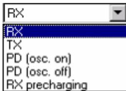
Leaving the crystal oscillator running gives a shorter turn-on time at the expense of higher current consumption in the power down mode. RX precharging can be used to reduce the demodulator turn-on time. Please refer to the data sheet for further information on demodulator precharging. The default value is RX.
