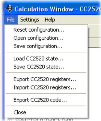
*Reset configuration*- This command will reset all fields in SmartRF® Studio. The connected device is not affected. The command is also available from the toolbar (white sheet).
