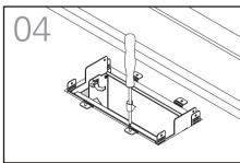
Use a Phillips head screwdriver to screw the tabs that you bent using the screws provided.
