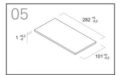
**CAP PLUS COVER LAYER:** To cover the Cap Plus cover with a finish that matches the desk (wood or another material), cut a layer with the same dimensions shown in figure 5.
