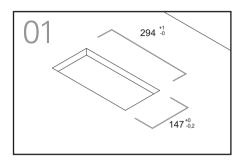
Cut an opening in the desk to recess the box with the measurements specified in figure 1.
