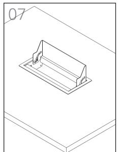
Check that the box cover opens perfectly to  $90^{\circ}$
