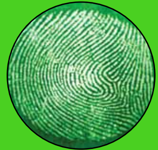
CYANOACRYLATE FUMED fingerprint on soda can photographed with a digital camera connected to the KRIMESITE™ IMAGER .
