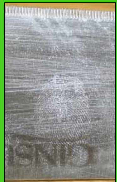
CYANOACRYLATE FUMED knife blade photographed in natural light—print faintly visible.
