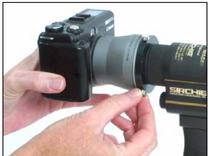
FIGURE 10 —Use the three thumbscrews to tighten the Camera Coupler to the eyepiece.
