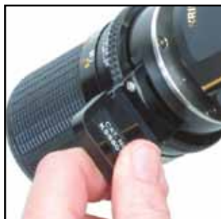
FIGURE 3—Always insert the sliding filter from the left side of the unit as shown, with label facing the eyepiece.
