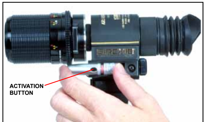
FIGURE 1—Snap the Laser Pointer into the mounting cradle located on the left side of the Imager.
