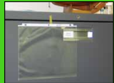
STEP 3 —Cover the suspected area with an 8.5" x 11" plastic sheet protector to protect potential trace DNA from shortwave UV light exposure.
