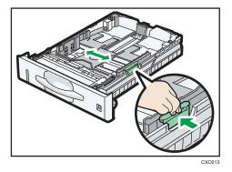
4. Pinch the end guide and slide it inward to match the standard size.
