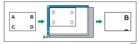
• Placing the original in the ADF
