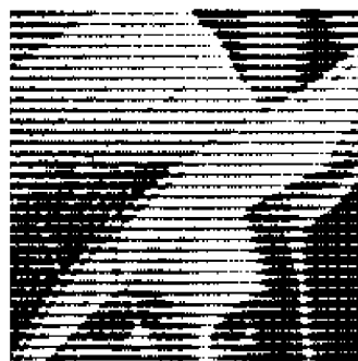
Figure 2.6 AM halftoned image using the threshold matrices shown above.
