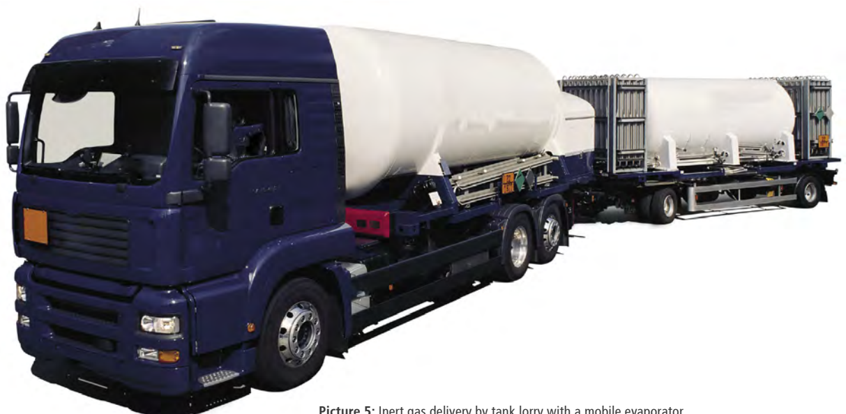
Picture 5: Inert gas delivery by tank lorry with a mobile evaporator
