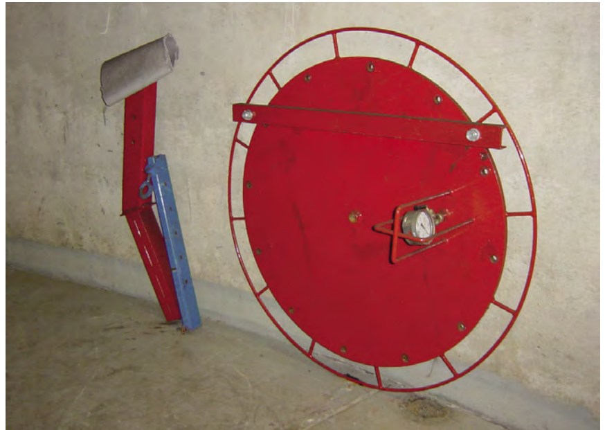
Picture 2: Prepared sealing for clearing-out of silo
