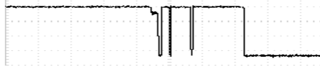
Figure 2: High-to-low switch transitory oscillations
