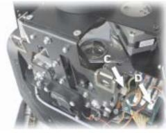
Once the frame with the Zoom/Focus mechanic unit has been removed, it is possible to clean the parts which are usually difficult to reach. Reassemble the Zoom/Focus unit carefully, being sure in particular that the blade with prism and frost is positioned between the two lenses of the Zoom/Focus unit. Remember then to connect again the 2 motors and the fan to their connectors.
