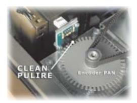
The sensors of the encoders concerning the PAN and TILT movements are located in the base and in the arm of the MP700 Zoom respectively. The pictures clearly show how you can reach these components and where you can correctly operate for their maintenance.
