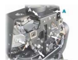
To make an extraordinary maintenance, it is necessary the presence of a generic or qualified mechanical operator, according to the type of the needed intervention. In order to make its use easier, we advise you to completely draw out the mechanic unit of the zoom and focus movements as follows: disconnect the two motors (connectors B and C) and the fan (connector D); remove the 4
