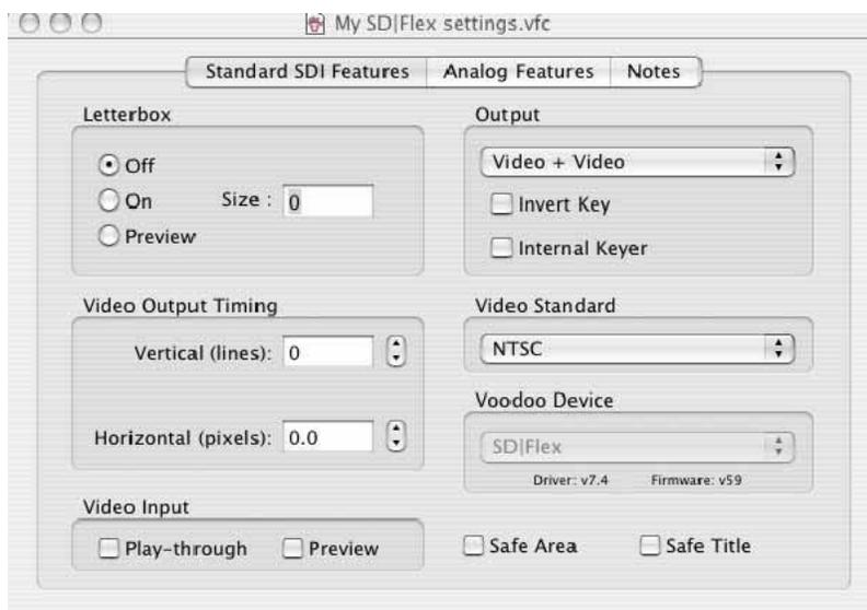
The Feature Control is the control interface that runs independently to the applications using the Video card.
