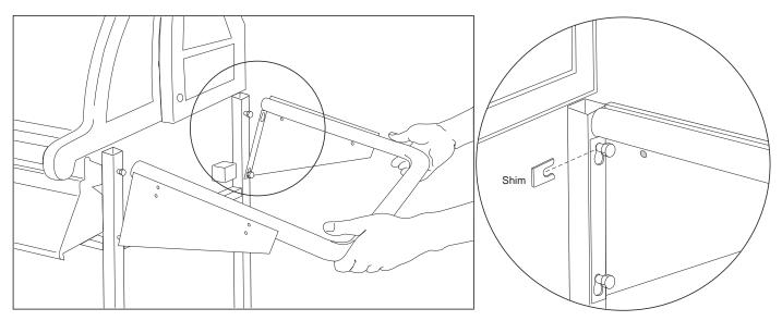
Attach the right shelf support to the barbecue by loosening the 4 existing leg bolts, approximately 3 turns only, so that the shelf support can slide over the bolt heads. Insert a shim washer sideways behind the head of one of the bolts and in front of the shelf support. Tighten the bolt using the 7/16" (11 mm) wrench/ratchet or adjustable wrench. Repeat inserting shim washers behind the heads of the remaining 3 bolts.
