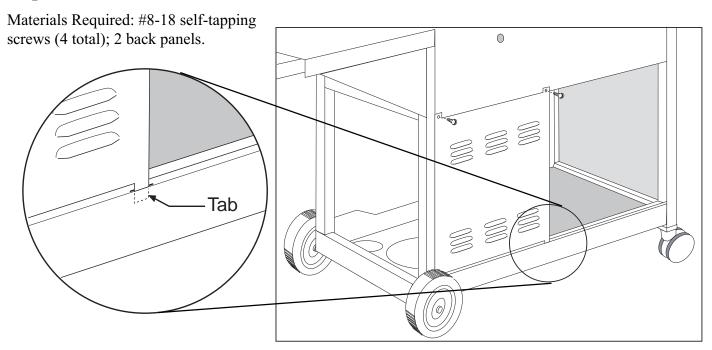
Place a back panel with the louvers facing down and to the rear on top of the rear leg brace. Ensure that the tab, the small flange on the bottom of the back panel, is inserted into the slits provided on the top edge of the rear leg brace. Secure the top of the panel using two self-tapping screws in the holes provided at the top right and left hand corner of the panel.
