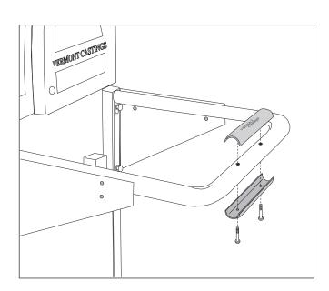
Place the top half of one handle grip, the half bearing the Vermont Castings logo, onto the right shelf support handle. Use the holes provided as a guide. Snap the two halves of the handle grip together and secure them using two Philips screws and a Philips screwdriver.
