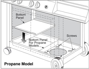
Insert the bottom panels of the cabinet by placing the lips of the panels on the front and rear leg brace. For Propane Models, the panel with the holes is to be placed on the right and secured with four self-tapping screws.
