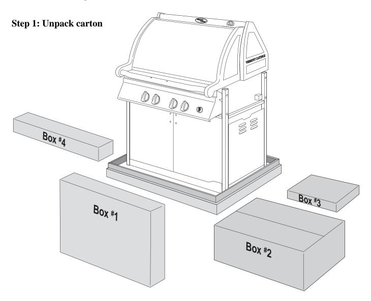
Use the knife or scissors to cut the strapping on the package then lift off the cardboard cap. Remove the cardboard sleeve lifting it straight over top of the barbecue. Check the 4 enclosed parts kits, against the parts list (Appendix A) to ensure that no parts are missing.
