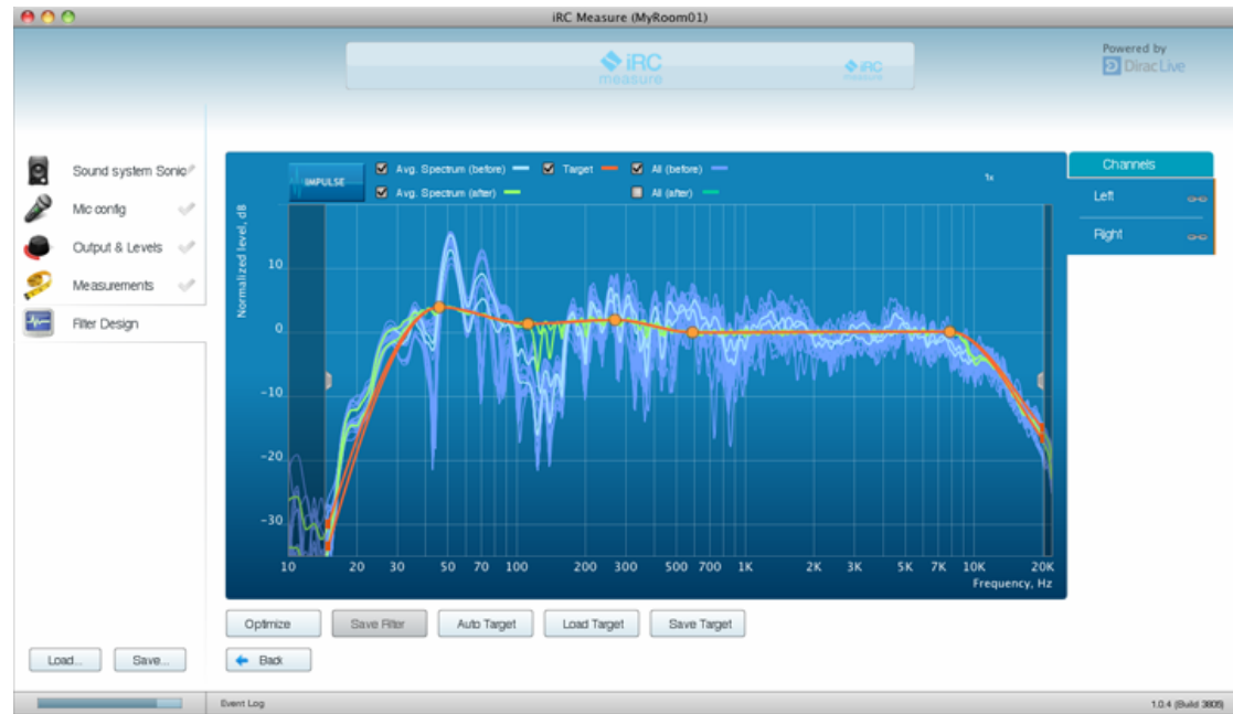
The iRC Measure app's Filter Design Tab. Note the wide frequency correction spectrum
