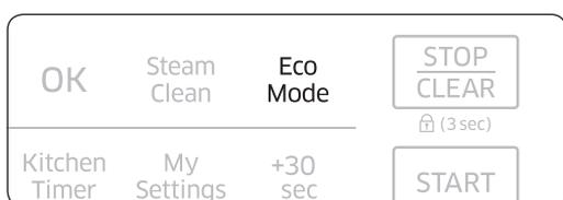
Eco Mode reduces standby power usage. When you press the **Eco Mode** button once, the display will go out and the microwave shifts to a mode which minimizes power usage. To cancel the Eco Mode, press the **Eco Mode** button once again, or press any other button.
