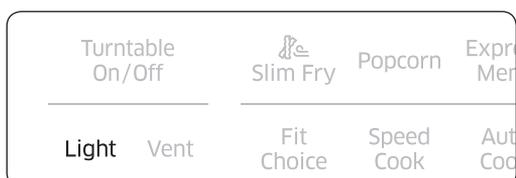
Press the **Light** button to turn the cooktop lamp on or off. Press the button once for high, twice for low, and three times to turn the cooktop lamp off.
