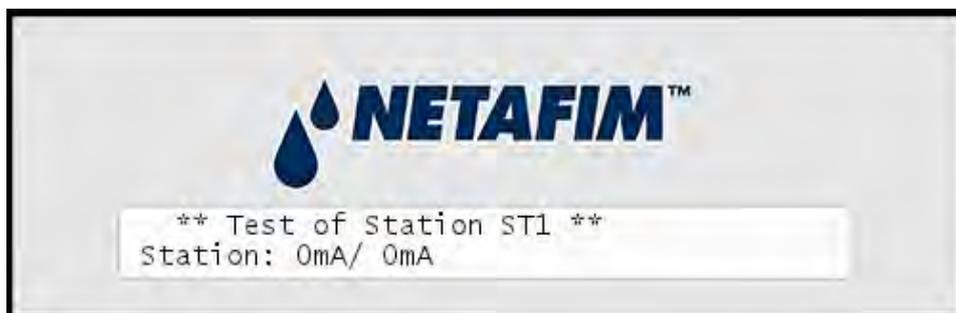
If the station is not working correctly it is typically not pulling any current at all - the current reading is 0 mA.
