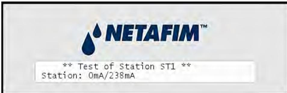
In this case the station is pulling a current of 238mA to keep the valve open, which is ok since this is typically in the 200-400 mA range.
