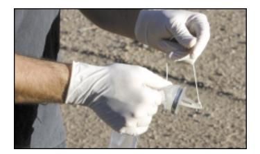
First, squeeze the full sampler just below the rigid plastic top ring to expel water resting above the flexible check valve. (Photo 1, top left)
