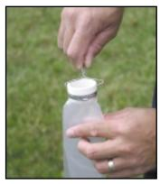
Attach the large clip by inserting the prongs into the holes at the top of the sampler.
