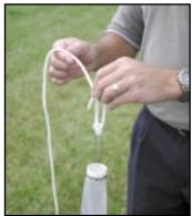
**5** Attach the suspension line to the upper clip. Tie securely.
