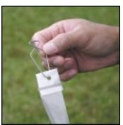
2 Slide the clip around so that the open end with the prongs faces away from the sample sleeve.
