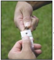
Remove sleeve and the 2 clips from package and unroll the sampler. Attach the small clip by inserting the prongs into the hole at the bottom of the sampler.
