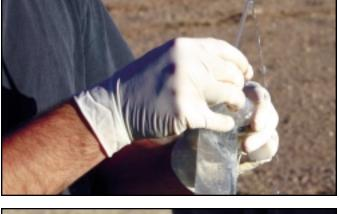
Raising and lowering the bottom of the sampler or pinching the sample sleeve just below the discharge tube will control the flow of the sample. The sample sleeve can also be squeezed, forcing fluid up through the discharge tube, similar to squeezing a tube of toothpaste. With a little practice, and using a flat surface to set the sample containers on, HydraSleeve sampling becomes a one-person operation.
