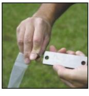
**3** Attach the reusable weight to the clip at the bottom of the sampler.
