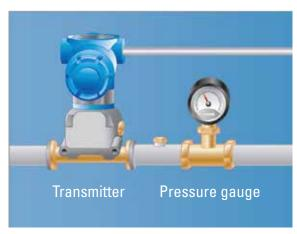
Figure 6: Pressure transmitters convert signals from pressure sensors
