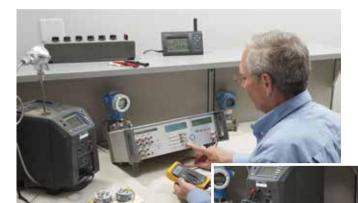
Figures 1 and 1a: A pressure calibration system needs to accurately measure pressure and may also need to measure pressure transmitters.
