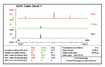
Figure 5: Offline VLF cable PD mapping with the Cable Data Collector.
