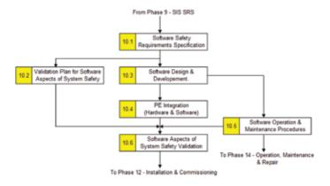
Figure 2: Realisation Phase - Software Safety Lifecycle.
