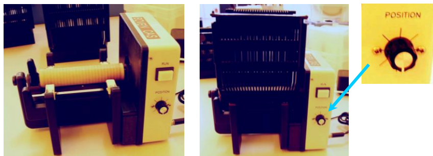
Fig.10: Wafer flat aligner; for the STS ASE tool select the down position .
