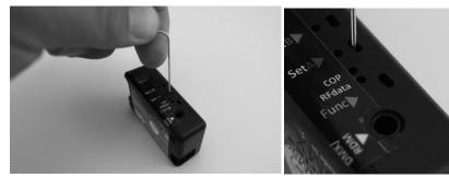
**Pressing SetA on an RC4 Series 3 DMX2dim.** The DimA indicator is behind the round hole. The button is behind the slotted hole. With a DMX channel set higher than 20%, press the SetA button and the DimA indicator will come on. Dimmer A is now assigned to that channel. It remembers this setting until you change it by pressing the button again.
