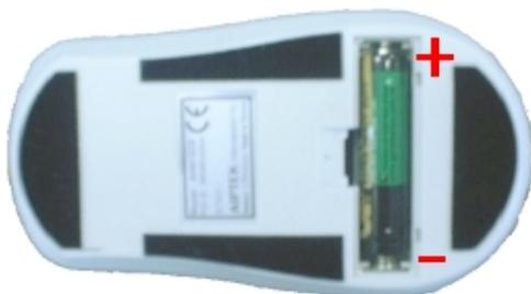
Figure 2b: inserting battery
