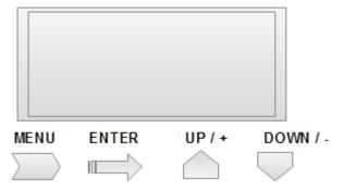
Turn on the main power, press "MENU" entering into main MENU, press "UP"/"DOWN" (+/-) to choose sub-menu, then press "SETUP".
