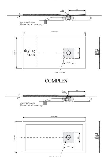
NOTE: All our Solidstone shower-trays are designed with a light inclination (not normalized) from 1400 where starts the drying area.
