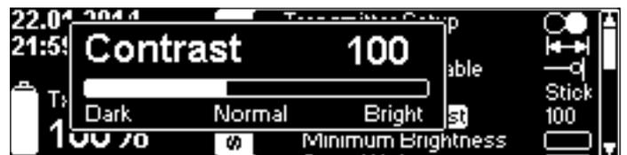
**Minimum Brightness** sets the low threshold for the ambient light sensor. The display will not go darker than the value set here. To save on battery life, use the lowest convenient value.
