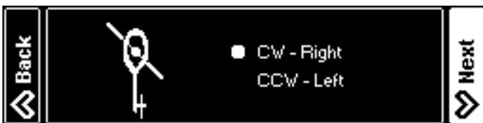
Select leading or trailing edge control depending on the layout of the rotor head.
