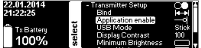
**USB Mode** allows to choose between **USB Stick** mode (for normal operation or setup/update purposes), **Simulator** (renders the VBar Control a USB game controller to go with your favorite simulator), or **No USB** (disables the USB connector temporarily).
