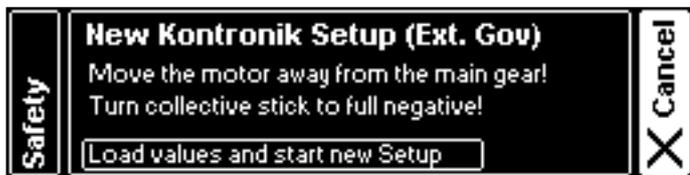
Move the collective stick to full negative to start with the ESC programming wizard. The screen will change so you can start the actual setup.
