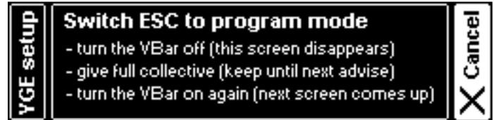
Your VBar Control transmitter and the VBar Flybarless Controller are in a programming mode now that allows you to program the ESC using the collective stick, as if it was connected to a regular receiver.
