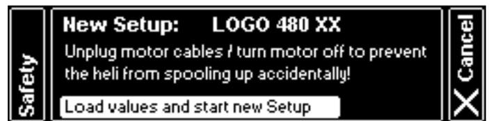
Select **Load values...** from the menu. This will load factory defaults for the LOGO series type and size into the VBar Flybarless Controller. Wait a few seconds for the process to finish.
