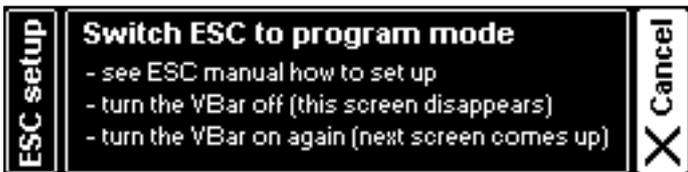
To enter the programming mode of the ESC, cut power to your VBar Flybarless Controller, and wait for the current screen to disappear. Now turn on your VBar Flybarless Controller again.
