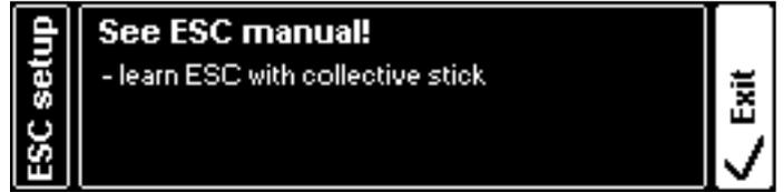
Your VBar Control transmitter and the VBar Flybarless Controller are in a programming mode now, which allows you to program the ESC using the collective stick, as if it was connected to a regular receiver.
