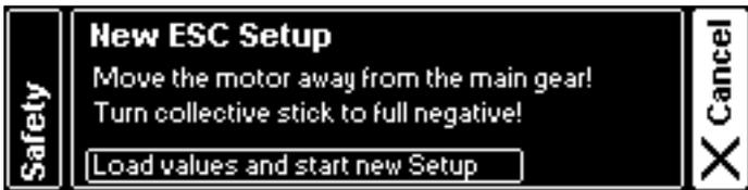
To start with the ESC programming wizard, move the collective stick to full negative. The screen will change so you can start the actual setup.
