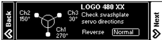
Use the trim controls to level the swash plate (90° to the main shaft for aileron and elevator, good visual judgment is precise enough) and to set it to the center of it's available collective throw. Make sure the servo arms are truly at 90° to the servos/links now. If not, adjust the links to the swash plate by the same amount, and/or move servo arms to achieve the least necessary electronic trim.
