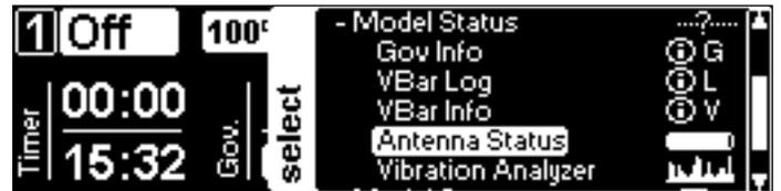
Once a VBar Control Satellite Receiver is connected, you can check the antenna status at **Model Status/Antenna Status**. You will see bars indicating the overall link power as well as the signal strength of the four antennae (Tx=radio, Rx=receiver).
