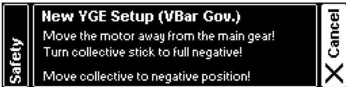
To start with the ESC programming wizard, move the collective stick to full negative. The screen will change so you can start the actual setup.
