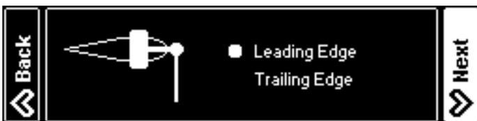
**Attention** If you have a heli with levers in between the rods from the swash plate to the blade grips, which reverse the direction of movement of the rods (seen e.g. on some TT helis), please set this parameter opposing to the display here, else some of the feed forwards (like tail rotor pre-compensation) might work the wrong way.
