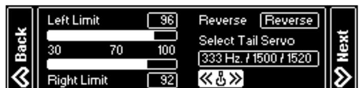
**Only now** connect the servo to the VBar Flybarless Controller and mount the servo arm as close to 90° as possible to the servo/tail push rod. The final trim will be done by the Autotrim feature (see page 32). For optimum performance, 90° angles should apply from the servo arm to the push rod and from the push rod to the bell crank on the tail gear box. This can be adjusted properly with the heli turned off, so you can move the servo arm and push rod manually.
