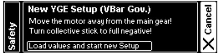
To enter the programming mode of the ESC, cut power to your VBar Flybarless Controller, wait for the current screen to disappear. Move the collective stick to full positive. Now turn on your VBar Flybarless Controller again.
