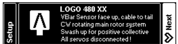
Connect the swash plate servos according to the graphics shown in the Wizard (nose of the model pointing away from you). In case you encounter issues with the control directions later on, double check proper connection of the servos again. Now mount the servo arms as close to 90° as possible to the servos/links. Connect the links to the swash plate.
