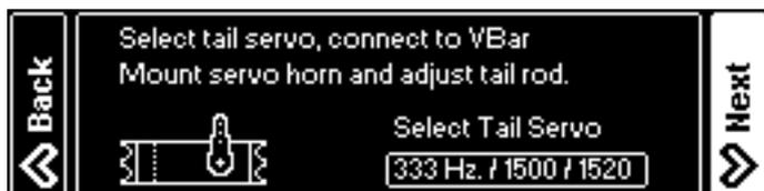
**Only now** connect the servo to the VBar Flybarless Controller and mount the servo arm as close to 90° as possible to the servo/tail push rod. The final trim will be done by the Autotrim feature (see page 32). For optimum performance, 90° angles should apply from the servo arm to the push rod and from the push rod to the bell crank on the tail gear
