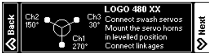
Check if the swash plate is moving correctly according to the stick inputs. If not, reverse. All three swash plate servos will be reversed simultaneously.
