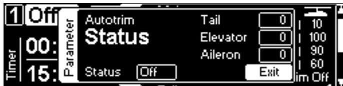
Autotrim activates the automatic trim feature of your VBar Flybarless controller. If enabled, the VBar will automatically trim the swash plate and the tail when the following conditions are met: the motor must be running, collective must be in the range for hovering, and the cyclic and tail sticks must be left alone.
