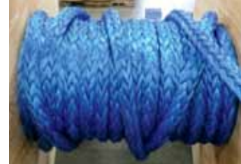
CROSS WINDING Second Cross
