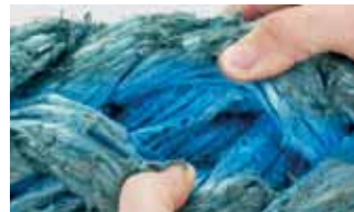
Inspect for internal abrasion.
