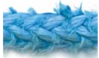
Severely abraded rope.
