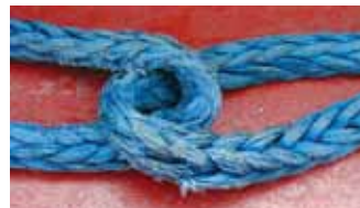
Eye-to-eye splice connection.
