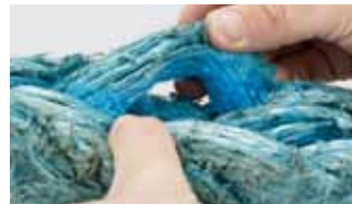
Inspect for pulled strands.
