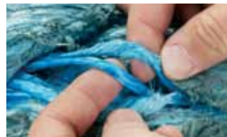
Compare surface yarns with internal yarns.
