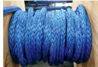
CROSS WINDING Level Layer
