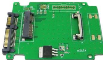
mSATA (mini-SATA) drives can be connected using the adapter shown above. This mSATA adapter connects to the SAS/SATA Extension Adapter.
