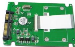
1.8" ZIF Drives can be connected using the adapter shown above. This ZIF adapter connects to the SAS/SATA Extension Adapter.
