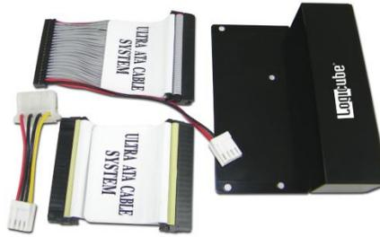
3.5" and 2.5" PATA/IDE drives can be connected using the 3.5" adapter shown above. The 3.5" adapter connects to the SATA/SAS Extension Adapter.
