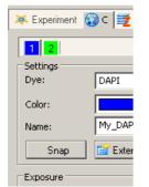
If you have a manual microscope then select the first channel (e.g.  $My\_DAPI$ ), set up your microscope for DAPI and click on the **Snap** button.
