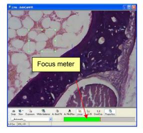
AxioCams also have a focus meter. Right click in the live image window to toggle between spot meter/focus bar on/off.
