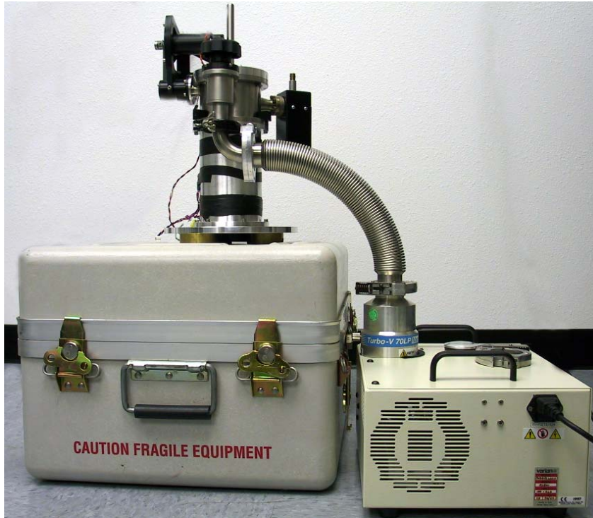
Figure 19. Turbo pump connected to dropping chamber. Note the minimum stress in the hose.
