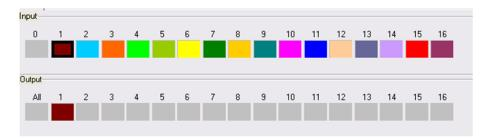
User can also set one input to more outputs. Click input channel 1 in Input area, and click output channel 1, 2, 3 in Output area, output 1, 2 3 will output signal 1, and the color of output channel 1, 2, 3 will corresponding to the color of input channel 1.
