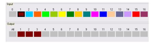
If need to close one output signal, for example, close output 3, click "0" in Input area, then click "3" in Output area, output 3 is closed, and turn to original gray.
