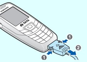
**Note:** Do not remove the battery from the phone without unplugging the adapter first. Otherwise, the phone may be damaged.
