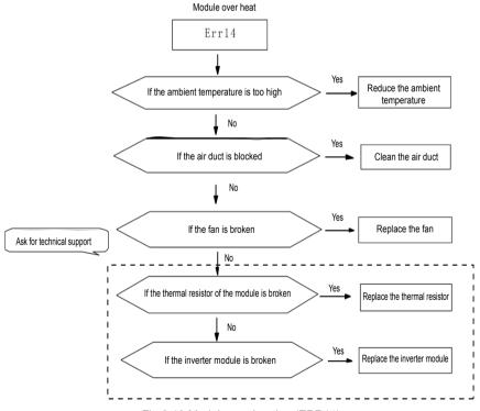
Fig.8-13 Module overheating (ERR14)
