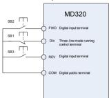
Fig.6-7 Three-line Running Mode 1
