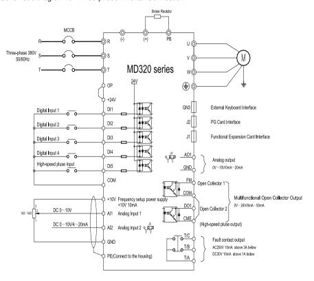
Fig. 3-6 Schematic Diagram for Three-phase Inverter Connection
