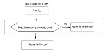
Fig.8-22 Earth short circuit fault(ERR23)
