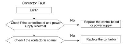
Fig.8-16 Contactor fault (Err17)
