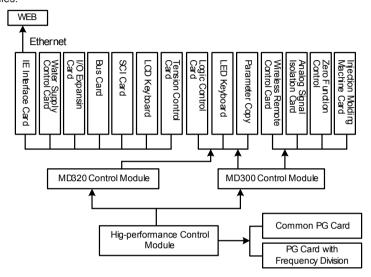
Fig. 2 MD Series Inverter Modular Structure Diagram
