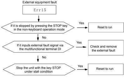
Fig.8-14 External equipment fault(ERR15)
