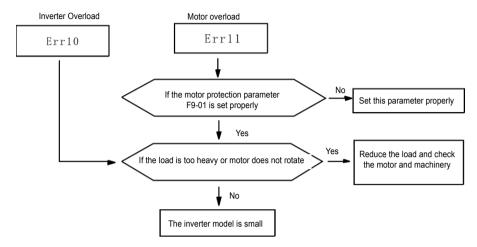
Fig.8-10 Inverter/Motor overload (ERR10/ERR11)
