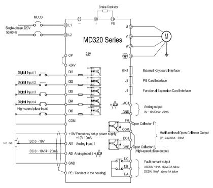
Fig.3-5 Schematic Diagram for Single-phase linverter Connection
