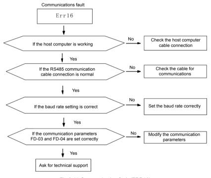
Fig.8-15 Communication fault (ERR16)
