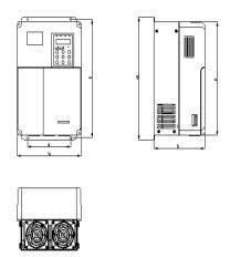
Fig. 2-6 Schematic Diagram for Physical Dimensions and Mounting Dimensions of 7.5kW  $\sim$  15kW
