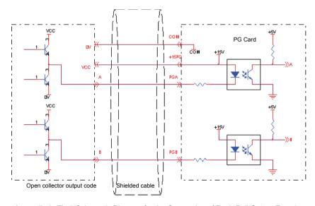
Appendix A: Fig.7 Schematic Diagram for the Connection of Push-Pull Output Encoder
