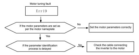
Fig.8-18 Motor tuning fault (ERR19)
