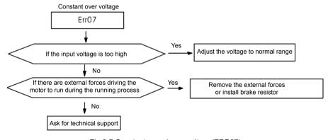
Fig.8-7 Constant speed over voltage(ERR07)
