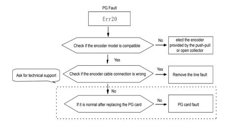
Fig.8-19 PG fault (ERR20)
