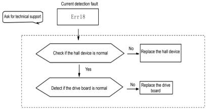
Fig.8-17 Current detection fault (ERR18)
