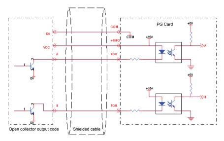
Appendix A: Fig.6 Schematic Diagram for the Connection of Collector Output Encoder
