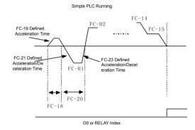
Fig.6-18 Schematic Diagram of Simple PLC
