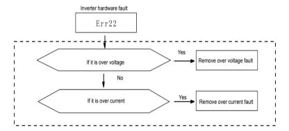
Fig.8-21 Inverter hardware fault(ERR22)
