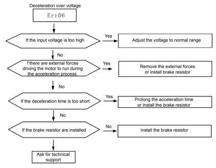
Fig.8-6 Deceleration over voltage (ERR06)
