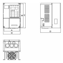
Fig. 2-5 Schematic Diagram for Physical Dimensions and Mounting Dimensions of 0.4kW  $\sim$  5.5kW
