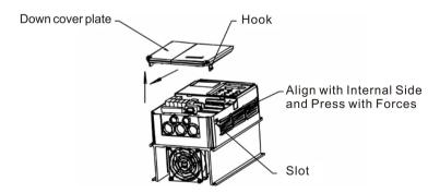
Fig.3-2 Removing the Lower Cover Plate of Plastic Enclosure
