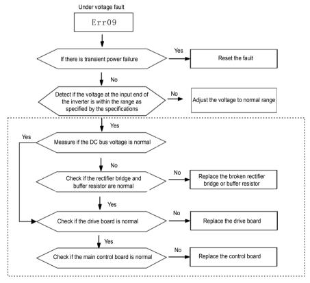
Fig.8-9 Under voltage fault(ERR09)
