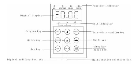
Fig.4-1 Operation Panel Diagram
