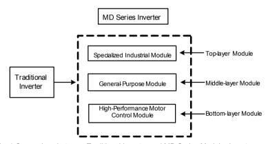
Fig. 1 Comparison between Traditional Inverter and MD Series Modular Inverter
