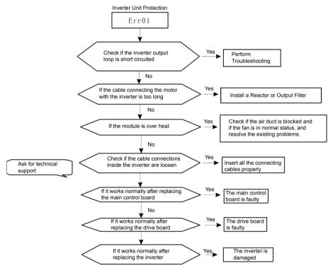
Fig.8-1 Inverter unit protection (ERR01)
