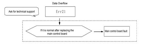
Fig.8-20 Data overflow (ERR21)
