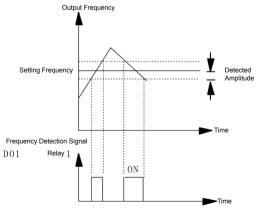
Fig.6-14 Schematic Diagram for Detection Amplitude
