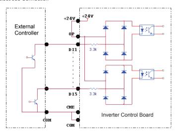
Fig.3-13 Source Electrode Connection
