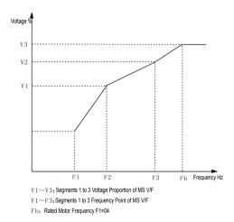
Fig.6-4 Schematic Diagram for V/F Curve Setup
