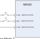
Fig.6-6 Three-line Running Mode 2
