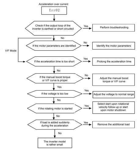
Fig.8-2 Acceleration over current (ERR02)
