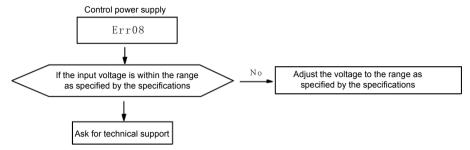
Fig.8-8 Control power supply fault(ERR08)
