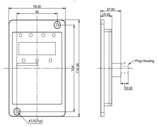
Fig.2-9 Schematic Diagram for Physical Dimensions of External Keyboard Mounting Hole Dimensions of External Keyboard
