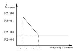
Fig.6-2 Schematic diagram of PI parameter
