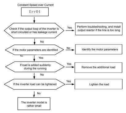
Fig.8-4 Constant speed over current (ERR04)
