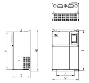
Fig. 2-7 Schematic Diagram for Physical Dimensions and Mounting Dimensions of 18.5kW  $\sim$  450kW
