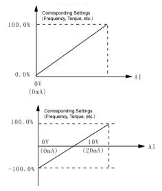
Fig.6-9 Corresponding Relationship between Analog Reference and Setting
