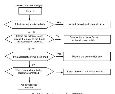
Fig.8-5 Acceleration over voltage(ERR05)
