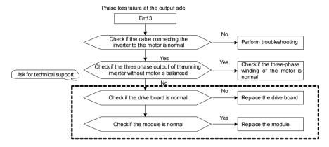
Fig.8-12 Phase failure at output side(ERR13)
