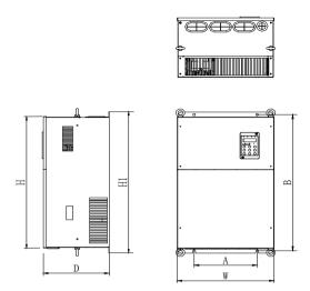
Fig. 2-8 MD320N Series Schematic Diagram for Physical Dimensions and Mounting Dimensions of 18.5kW  $\sim\!$  450kW
