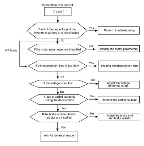
Fig.8-3 Deceleration over current (ERR03)
