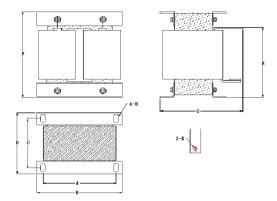
Fig. 2-11 Schematic Diagram for Dimensions of External reactor
