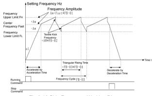
Fig.6-16 Skip Frequency Working Diagram
