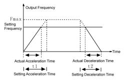
Fig.6-1 Schematic diagram for acceleration/deceleration time
