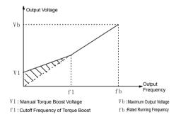
Fig.6-3 Schematic Diagram for Manual Torque Boost
