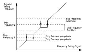
Fig.6-11 Schematic Diagram of Skip Frequency
