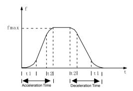
Fig.6-10 Schematic Diagram for S curve Acceleration/Deceleration
