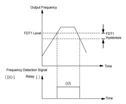
Fig.6-13 Schematic Diagram of FDT Level
