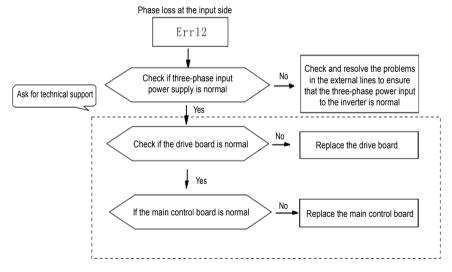
Fig.8-11 Phase loss at input side(ERR12)
