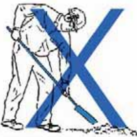
Figure 1: Poor shovelling technique. Extended reach forward.
