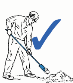
Figure 3: Shovel Type 1: Trench shovel with a flat blade.
