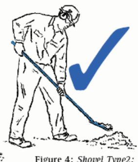
Figure 4: Shovel Type 2: Trench shovel with an angled blade.
