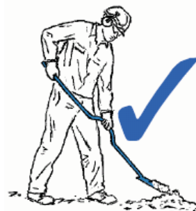
Figure 5: Trench shovel. A bend in the shaft to reduce forward bending.
