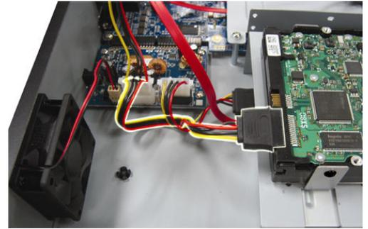
**Note:** Make sure the HDD power cable is connected to the **WHITE** jack on the DVR mainboard as shown below. The black jack is reserved for DVD writer installation.
