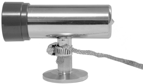
Figure 2-8 Grounding a Convectron Gauge
