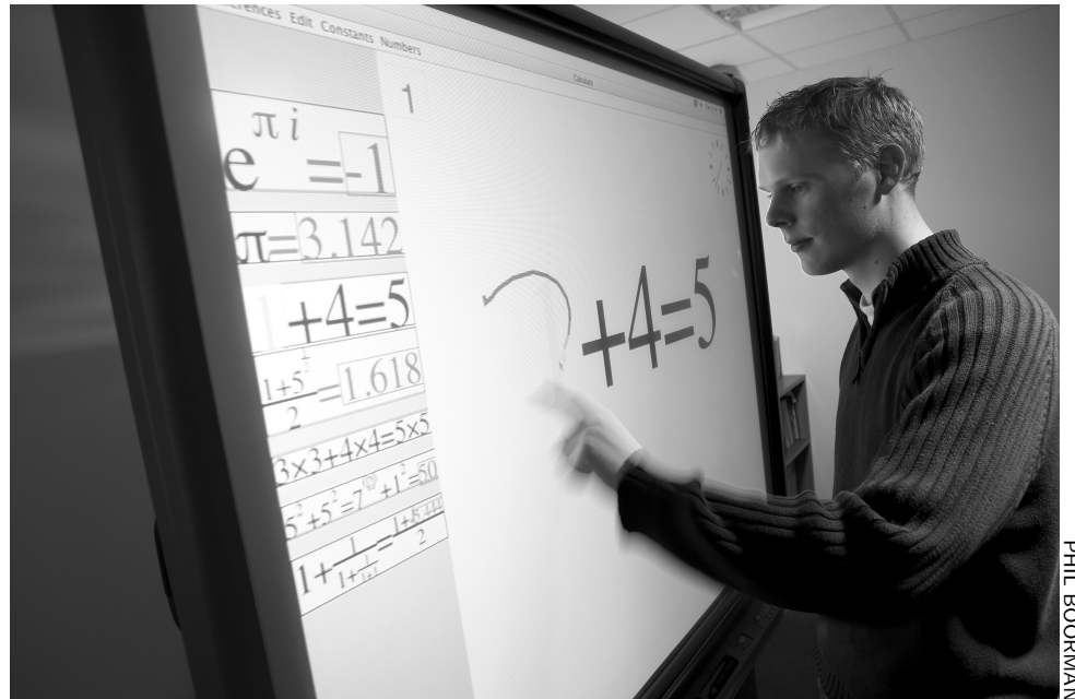
Figure 12.7: Writing on the new calculator using an interactive whiteboard. The whiteboard has a back-projection so the user does not cast a shadow on it, and it detects where they are writing by using cameras.
