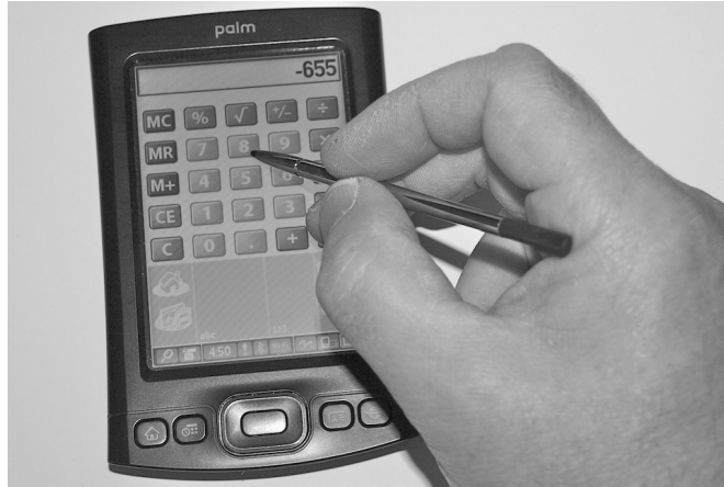
Figure 12.6: A PDA simulating a calculator. Instead of pressing buttons with your finger, a stylus is used on the touch-sensitive screen. Compare this with figure 3.1 (p. 62).
