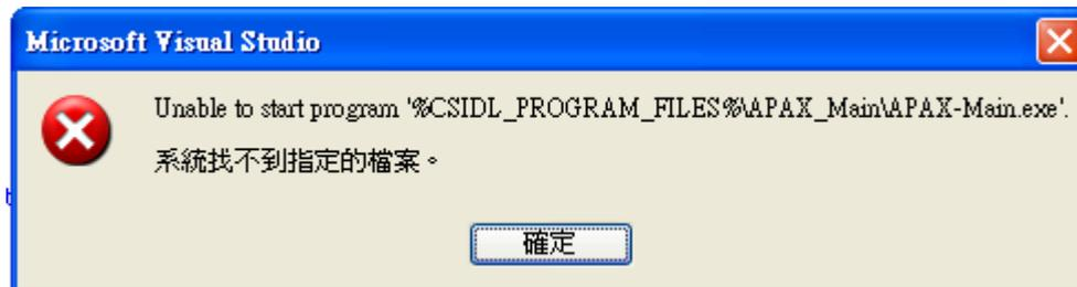
You can apply **Advantech DiagAnywhere** to transfer DLL files to program folder on target device. The program folder can be found under **Program Files**.
