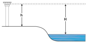
**h** height from the barometer installation to the reference point (for example: the runway).
