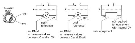
\* If necessary, use ferrite ring and twist pair wiring to reduce electrical interference.
