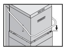
To avoid heat loss, lower hood to "Stand By" position between wash cycles.
