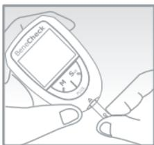
Fully insert the contact bar of the test strip into the test port of the meter. The meter will turn on automatically with test mode display and code number appear on the Screen.
