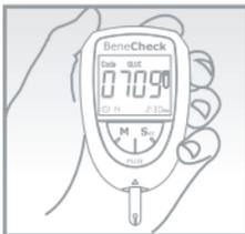
Insert a test strip into test port, the meter will turn on automatically.
