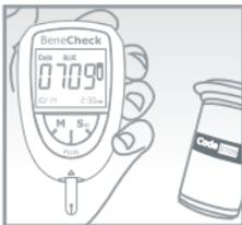
Check the test mode and code number on the screen are the same as the one on the test strip vial. Icon "GLUC", "UA" and "CHOL" indicate measuring mode of glucose, uric acid and total cholesterol respectively. If not, remove the test strip and recoding the meter is necessary as described in Section 2.3.
