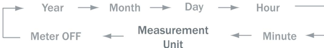
3. Click the right "Set" button for six times, and a blinking "mg/dL" will display on the screen.
